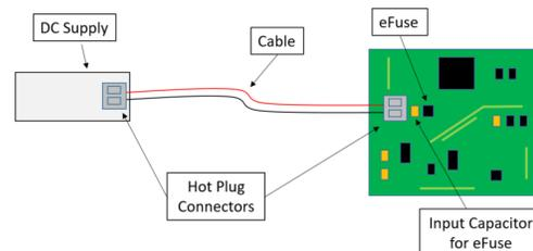
Figure 2. System Diagram
