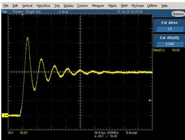
Figure 9. Lab Measurement with 1 μF Capacitor and an NIS5420 eFuse Connected in Parallel
