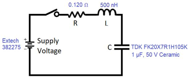
Figure 7. Lab Measurement Circuit
