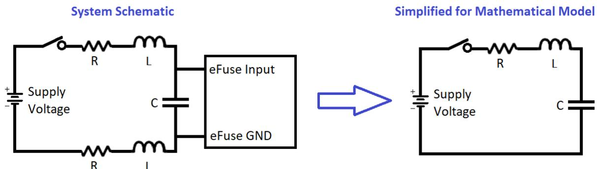
Figure 3. The System Schematic is Converted to a Simplified Series RLC Circuit since the eFuse can be Considered High Impedance. Also since the Positive and GND Return Cables are in Series they can be Lumped Together
