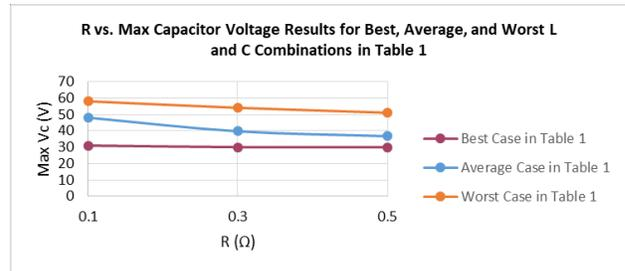
Figure 10. R vs. Average Max Capacitor Voltage
