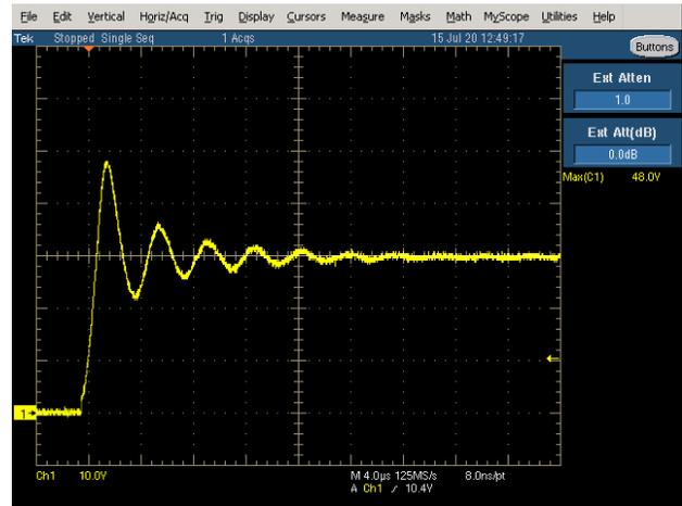
Figure 14. Voltage Spike was Reduced from 54 to 48 V with the Addition of the 33 V Zener Diode
