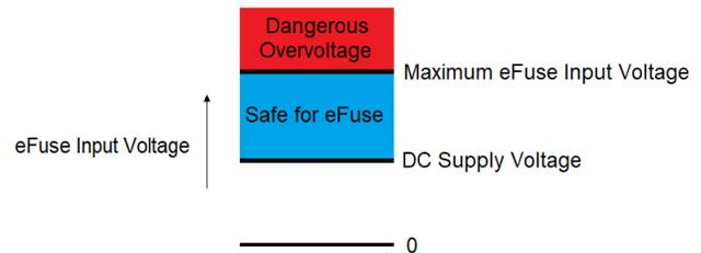
Figure 1. Important Voltage Levels in a System with an eFuse
