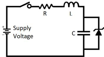
Figure 13. Addition of Zener Diode
