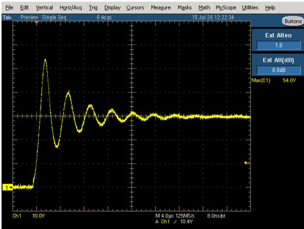
Figure 8. Lab Measurement Hot Plugging into a 1 μF Capacitor Only (no eFuse)
