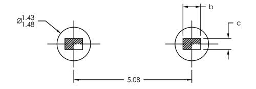
NOTE: LAND PATTERN AND THROUGH HOLE DIMENSIONS SERVE ONLY AS AN INITIAL GUIDE. END-USER PCB DESIGN RULES AND TOLERANCES SHOULD ALWAYS PREVAIL.
