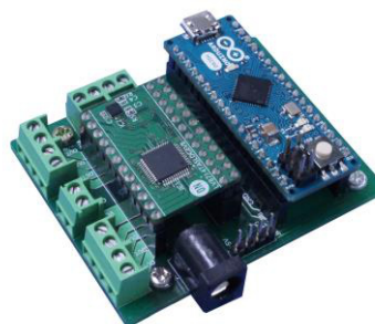
図 2. ONBB4AMGEVB Board with Arduino Micro and LV8714TASLDGEVB Board
