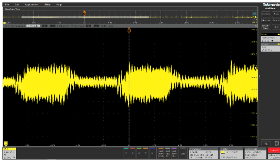
Figure 26. Transient Load on 12 V BUS
