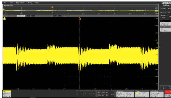
Figure 25. Transient Load on 9 V BUS
