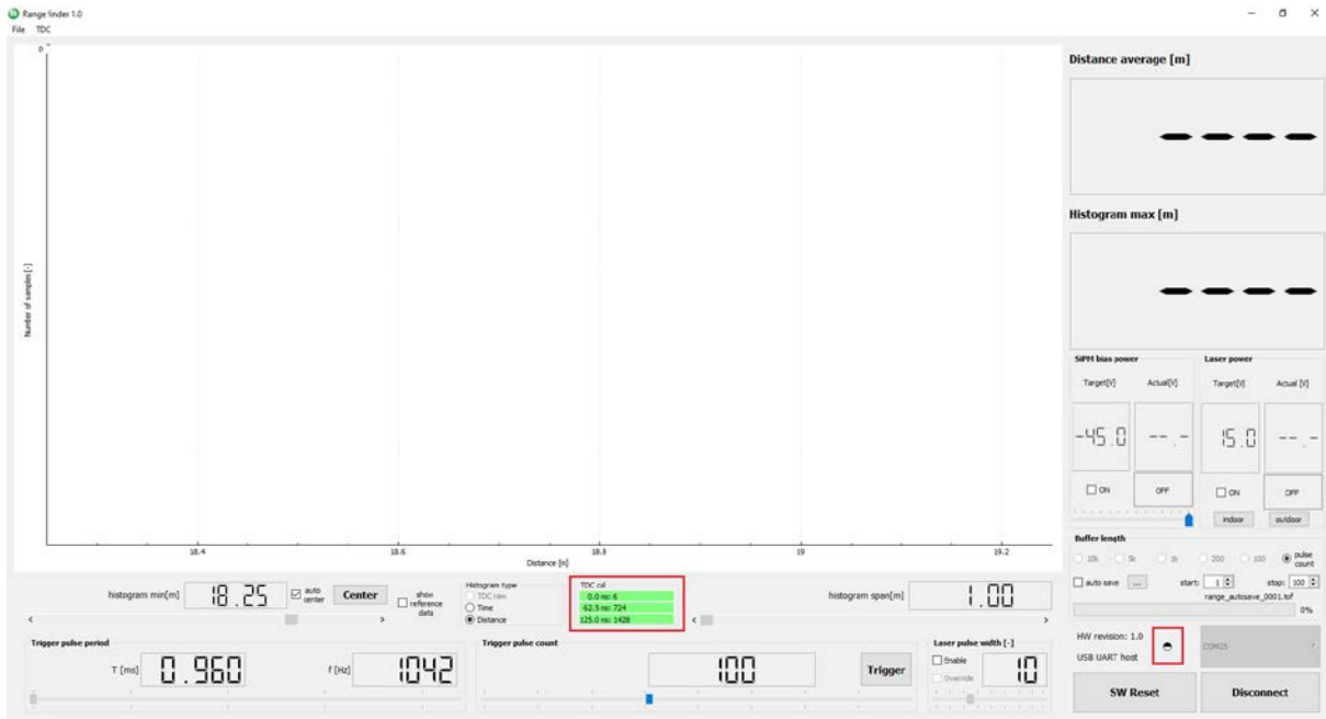
Figure 6. TDC calibrated automatically and application connected to LiDAR Platform
