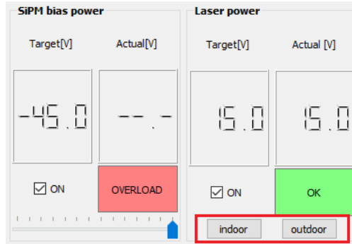
Figure 7. Overload Condition for Reference SiPM at high ambient illumination (outdoor)
