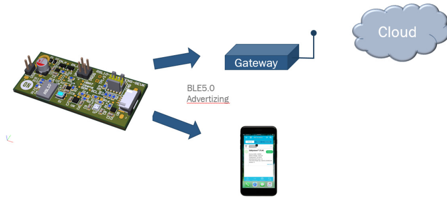
Figure 8. Complete System Outlook Including Sensor, Gateway and Cloud Service
